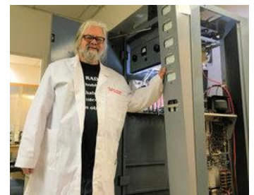
AM superstar Tim Smith, WA1HLR, with the Gates BC-1T AM broadcast transmitter he helped to restore for occasional use under W1AW or under the ARRL Headquarters Operators Club call sign, W1INF.
